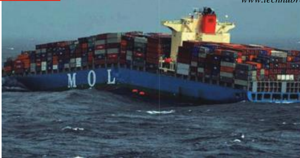
Figure.1. MOL Confort structural failure [16]
